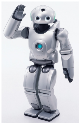
Fig. 2. QRIO, a small humanoid robot developed by Sony Corporation in 2003 which we use as a research platform.
