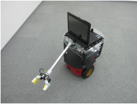
Figure 2: The slave robot that is remotely controlled by the operator child. It has one DOF gripper hand and a Skype monitor PC. The mobile base is built on Pioneer P3-DX whose movement is controlled by the encoder signals sent from the tricycle-style teleoperational interface.
