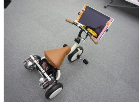
Figure 1: Tricycle-style teleoperational interface by which a child operator directly controls a remote slave robot (Figure 2). The operator can see a Skype monitor on a tablet PC and can also control the gripper hand of the robot.
