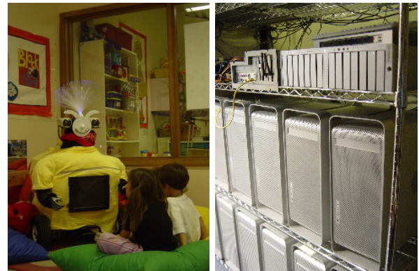
Fig. 5. Left: The appearance of RUBI is in constant change based on feedback from children and teachers. Two of the early critics were Kai and Marina Movellan. Right: RUBI's sensors send information to a 24 G5 Power PC cluster. The cluster is being used for experiments for RUBI to discover object categories from interaction with the environment [3].
